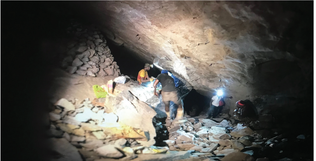
Figure 6 Chiselling an underground pillar. Tarkwa, March 2022.
