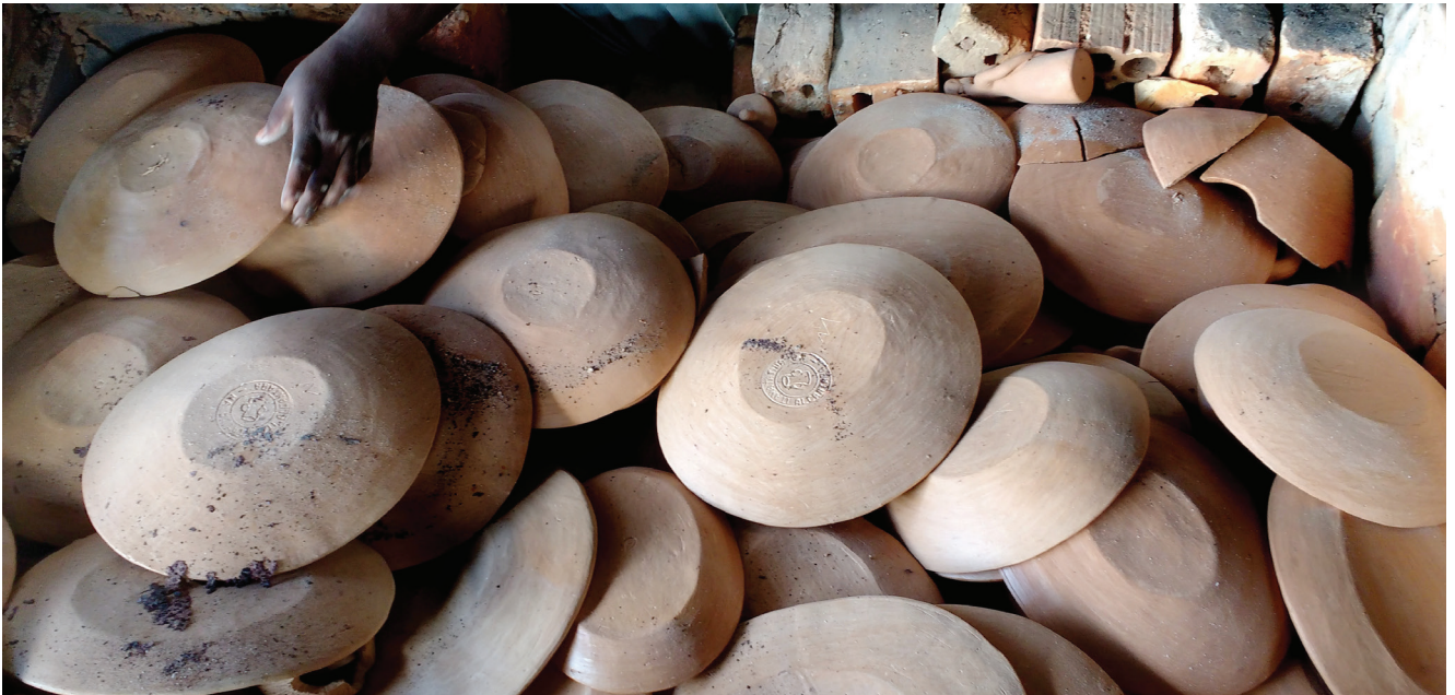
Figure 4 Plates being removed from the oven.
